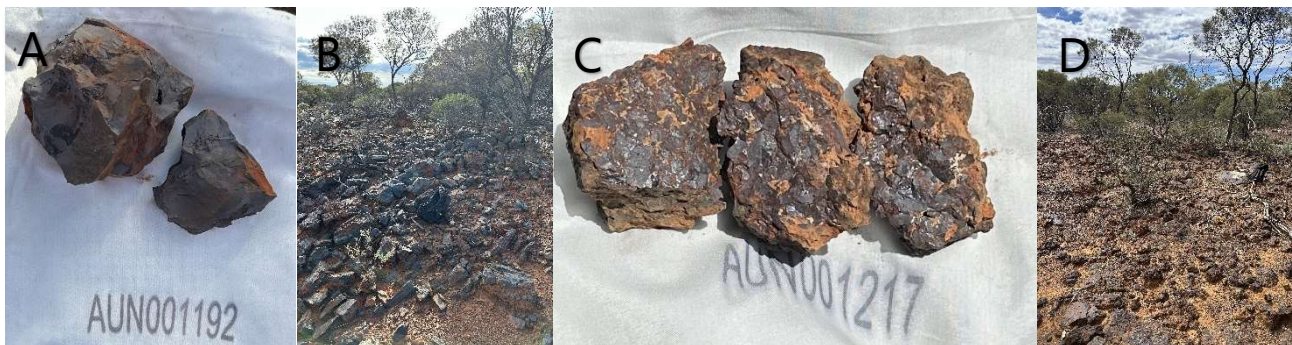
Figure 9. (A) Hematite enriched BID (Sample AUN001192 – 65.17% Fe), (B) outcropping hematite enriched BID, (C) hematite enriched capping / pisolite (Sample AUN001217 – 59.62% Fe), (D) outcropping cemented hematite pisolite potentially representing immature paleochannel iron deposits or capping. Results are presented in Annexure E.
