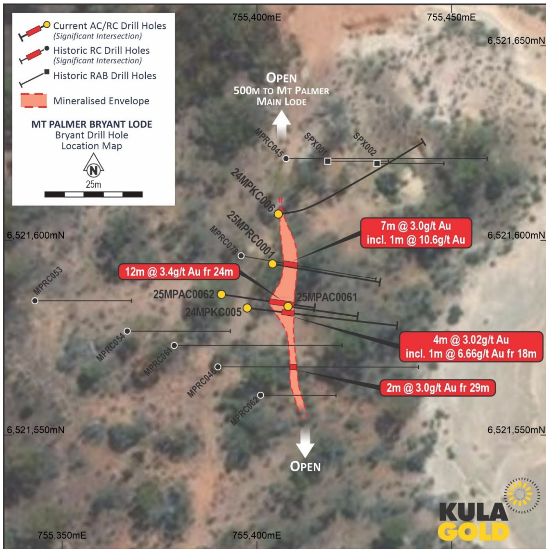
Figure 3. Mt Palmer Bryant's Lode plan view showing drill collars and mineralised envelope, which is open north, south and at depth.
