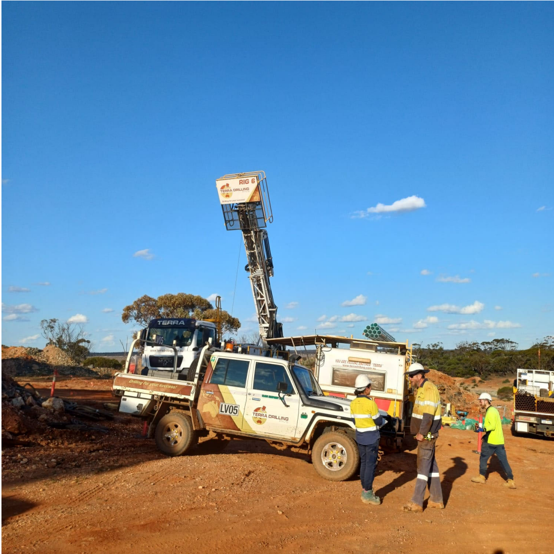
Figure 3: Diamond drill rig in operation at Mt Palmer with Terra Drilling and Kula personnel.
