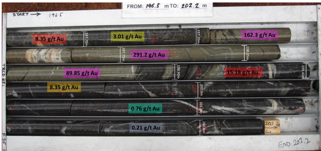
Figure 9 – Mineralised BIF core from Two Mile BIF domain. Historical TRY hole TRCD825 196.5m to 202.2m
